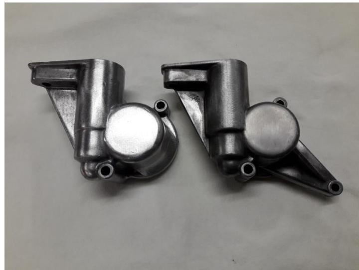
Bolt the angle housing, with a good oil seal, on to the adapter plate using the original bolts (serial number pointing down).
